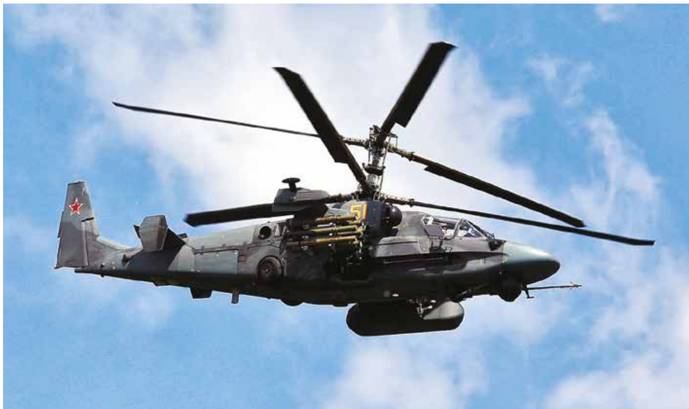
Ka-52 Alligator attack helicopters have distinctive double-rotors, side-mounted 30-millimeter cannons, and a dozen anti-tank guided missiles on stub wings.
