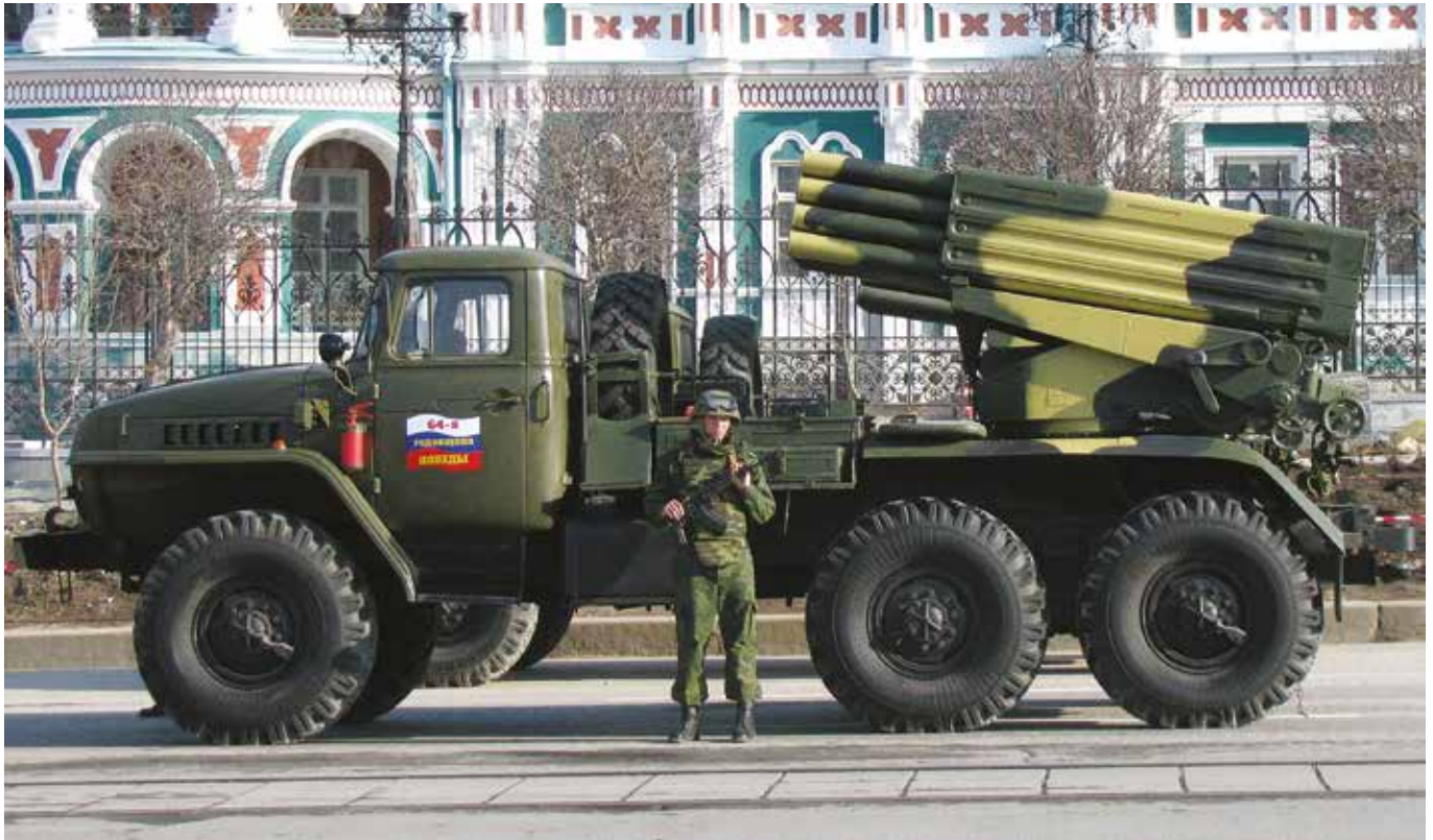
BM-21 is one of the multiple launch rocket systems used by the Russian army. One battalion of 18 launchers can deliver 720 rockets in a single volley.
